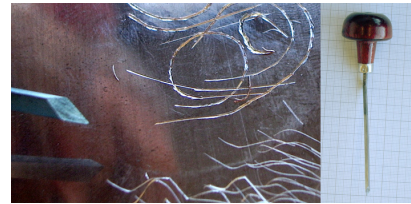
Figure 1: On the left a copper plate is being engraved with a "V" shaped burin and on the right the burin tool is shown.
